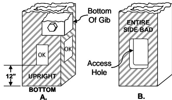
Figure 68 shows areas to avoid on the uprights of straight side machines of tie rod construction. The cross-hatched areas should be avoided.
