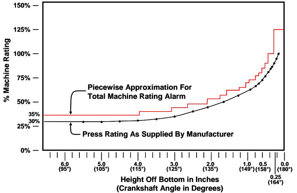
Figure 38: Example Tonnage De-rate Curve
