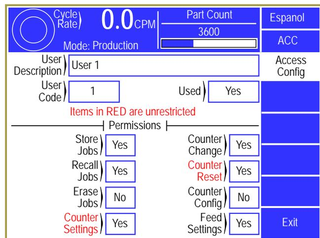
**Figure 42: User Access Configuration Screen**
