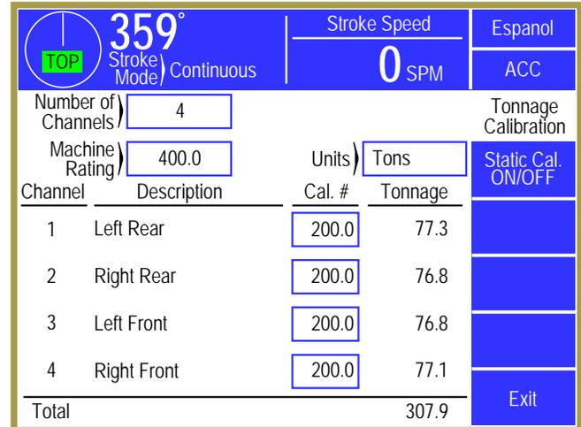
**Figure 36: Tonnage Monitor Tonnage Calibration Screen**
