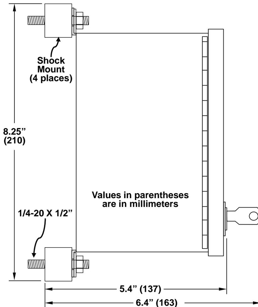
**Figure 51: Enclosure Dimensions Side View with Shock Mounts**
