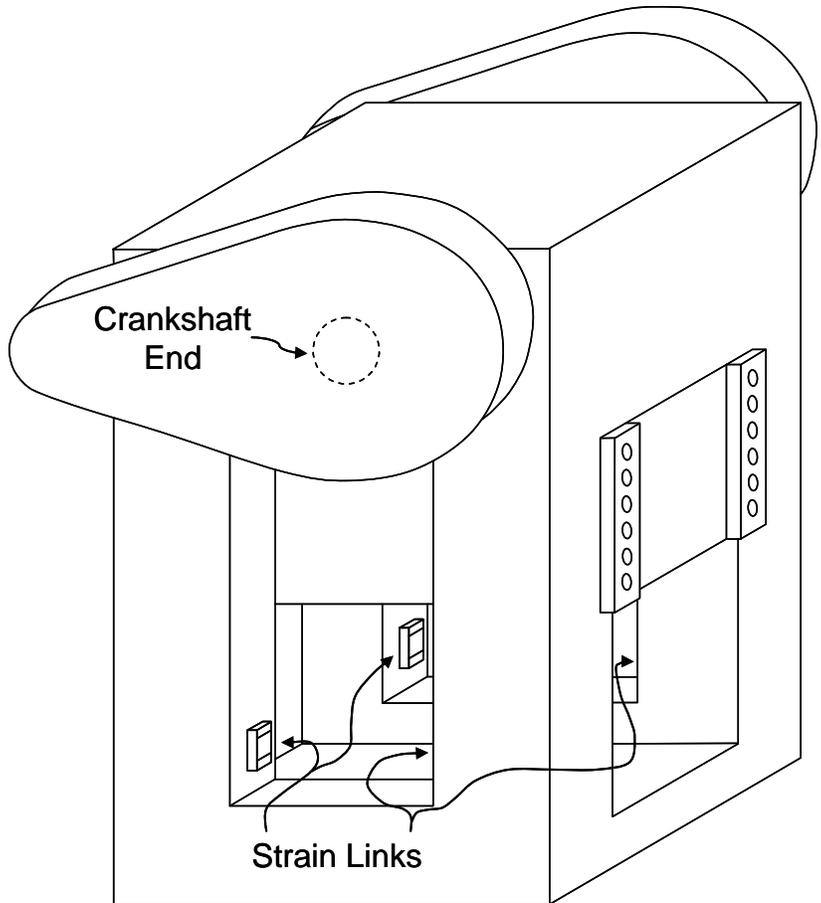
Figure 69: Solid Frame Machine Gage Locations
