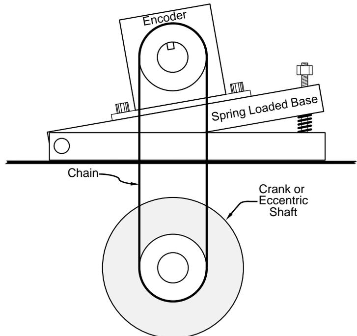
Figure 54: Encoder on Spring Base
