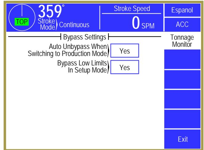
Figure 34: Bypass Settings Configuration Screen
