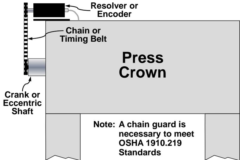
Figure 53: Resolver Mounting to Shaft
