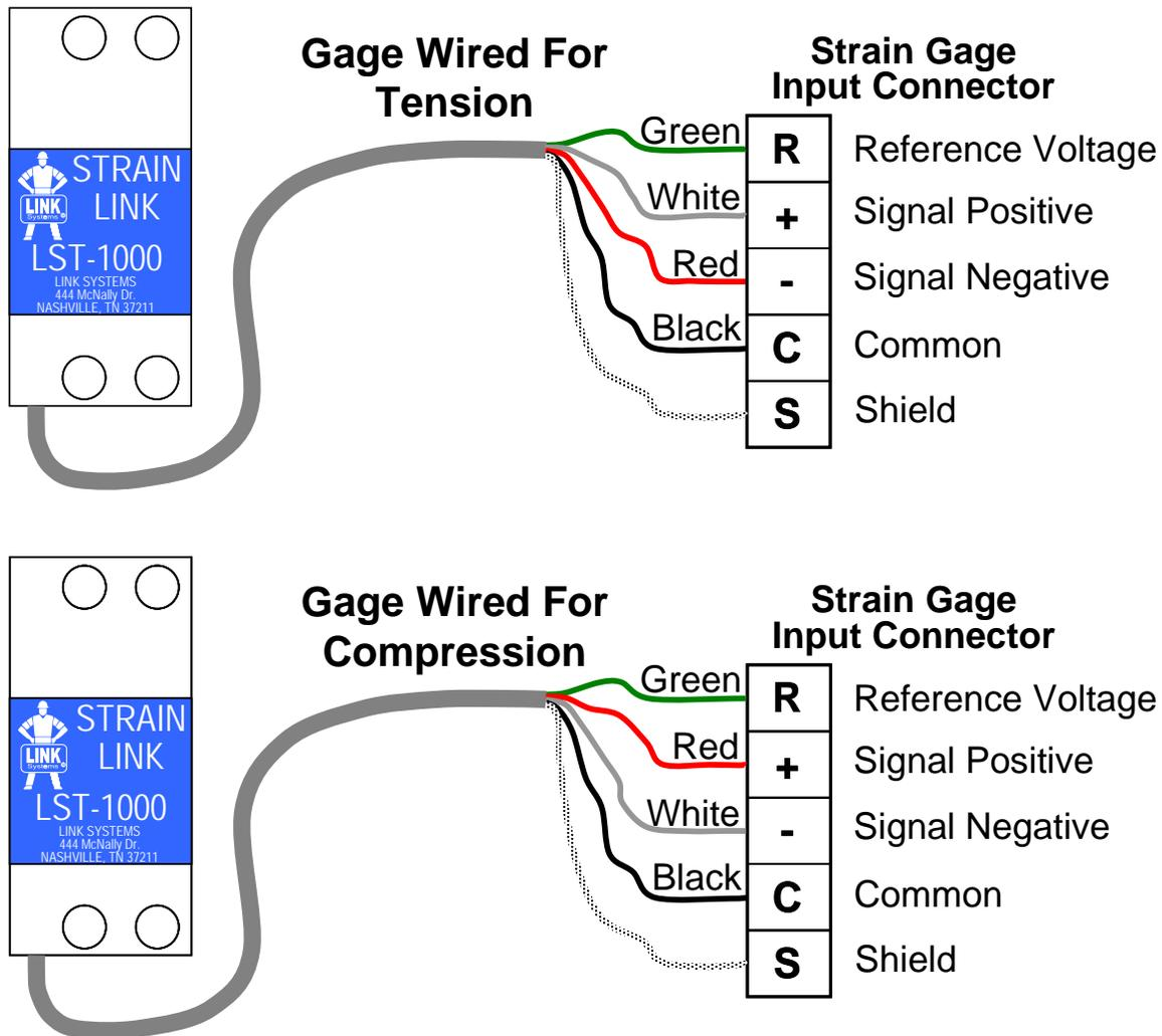
Figure 65: Strain Gage Wiring
