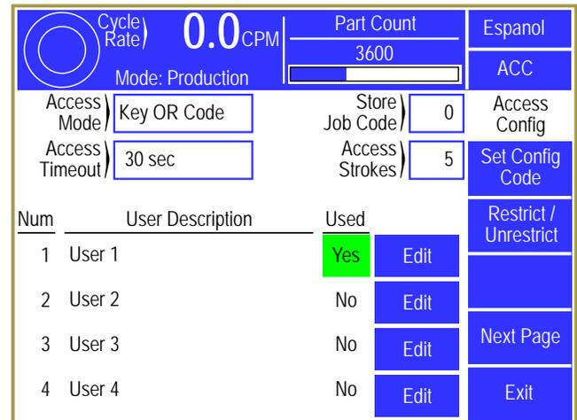
**Figure 41: Access Configuration Screen**
