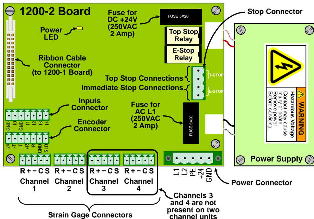
Figure 59: 1200-2 Board Connections
