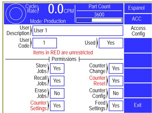
Figure 42: User Access Configuration Screen
