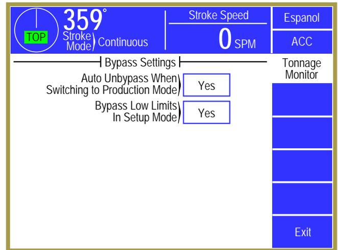
Figure 34: Bypass Settings Configuration Screen
