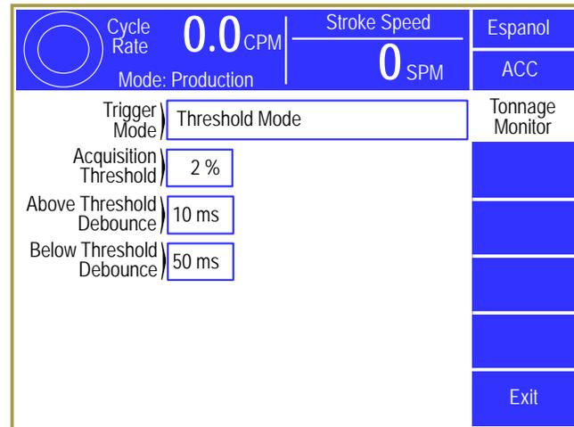
Figure 28: Threshold Trigger Mode Config
