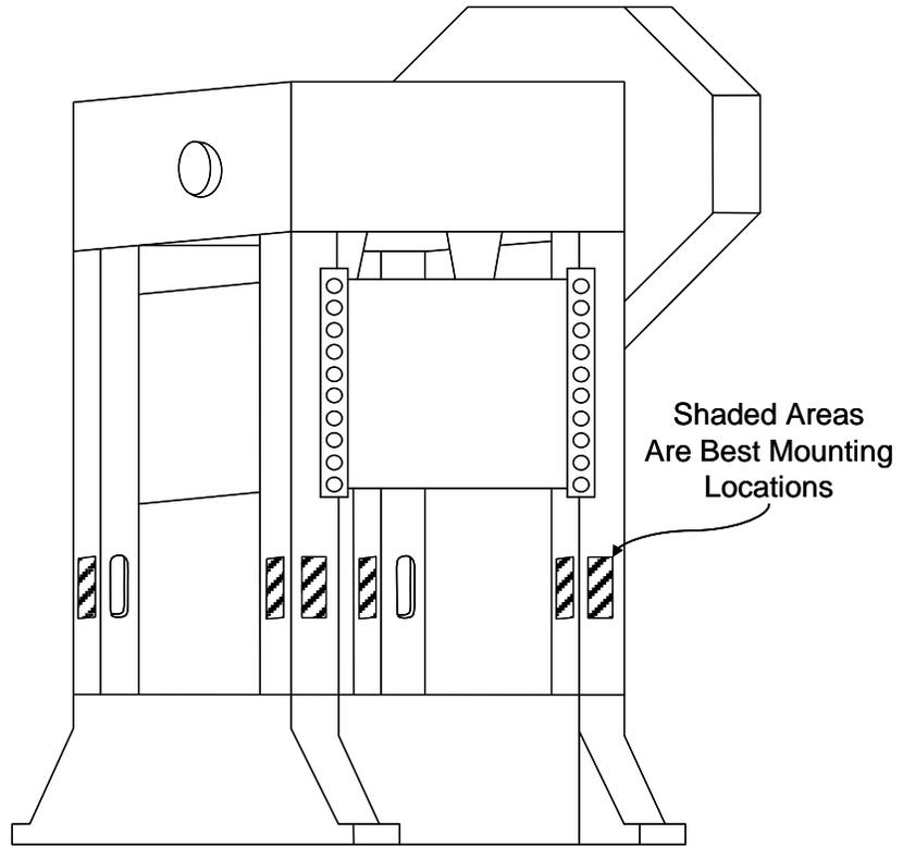
**Figure 67: Straight Side Machine Gage Locations**
