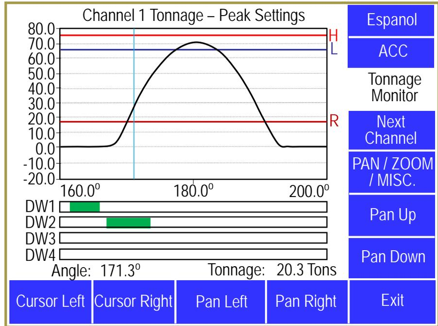
Figure 76: Load Cell Hit with Good Tie-Rod Tension
