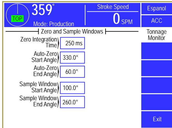
Figure 35: Zero and Sample Windows Configuration Screen
