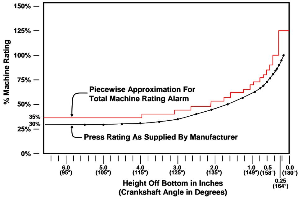
Figure 38: Example Tonnage De-rate Curve
