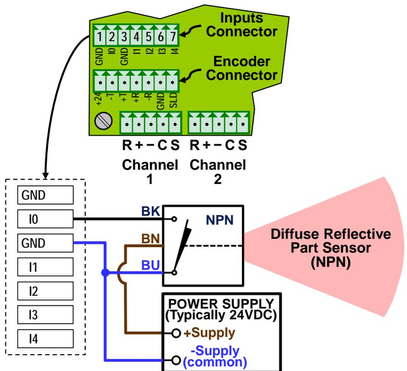
Figure 64: Inputs driven by NPN sensor
