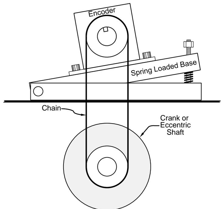
Figure 54: Encoder on Spring Base
