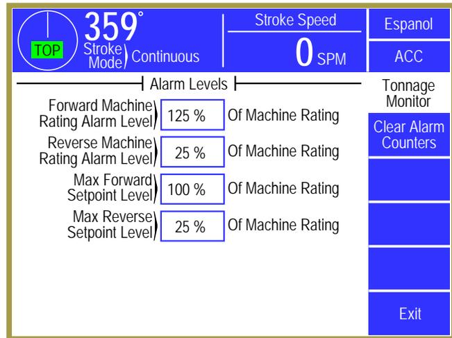
Figure 33: Alarm Levels Configuration Screen
