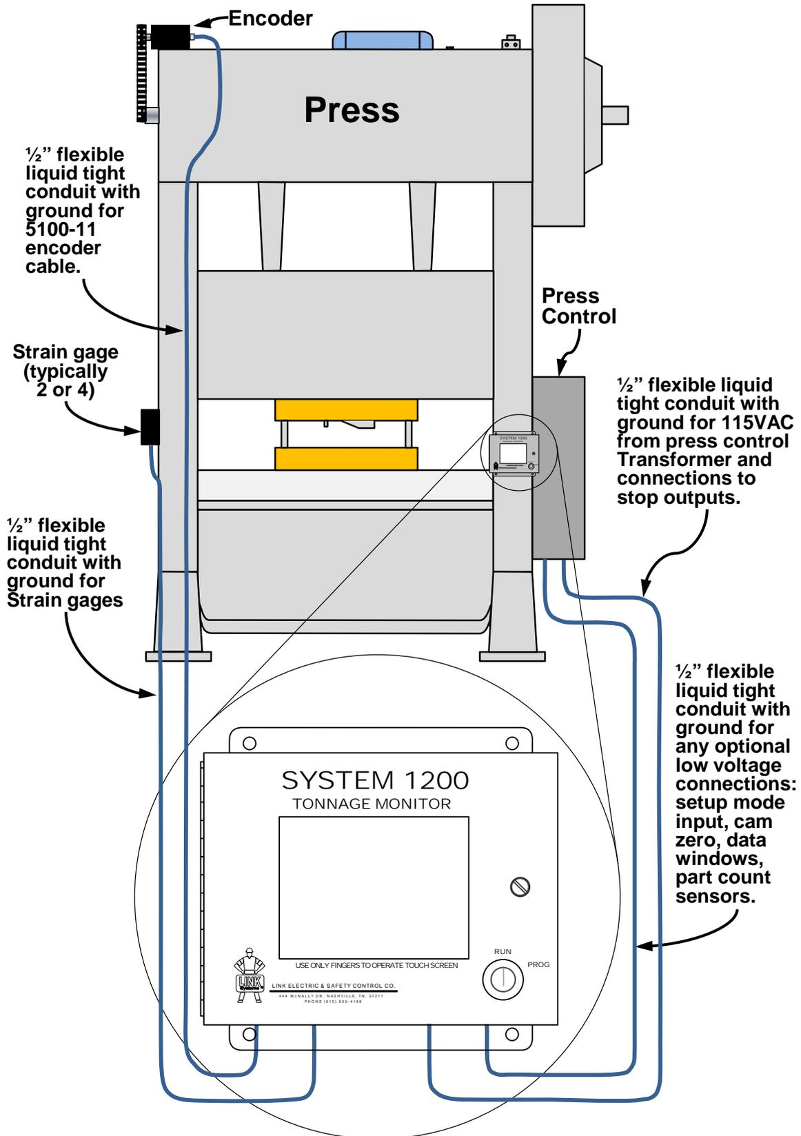
**Figure 58: General View of Wiring Runs for Installation**
