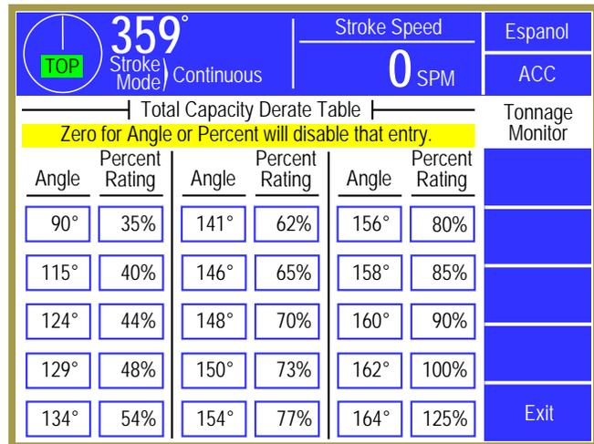
**Figure 37: Tonnage Monitor Total Capacity Derate Screen**
