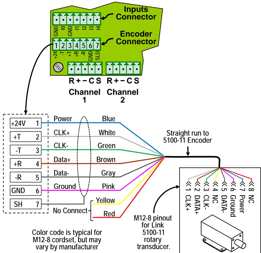
Figure 61: 5100-11 Encoder Connections
