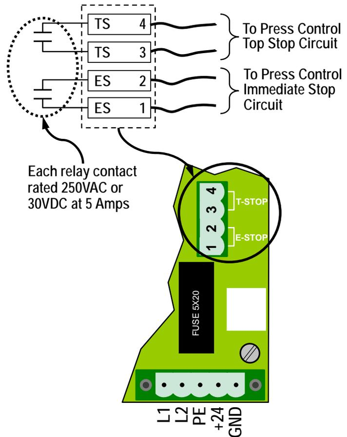
Figure 60: Breakaway of Stop Connector
