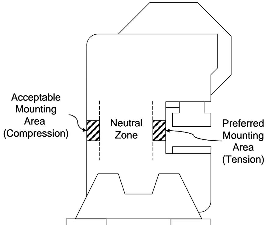
Figure 66: "C" Frame Machine Gage Locations
