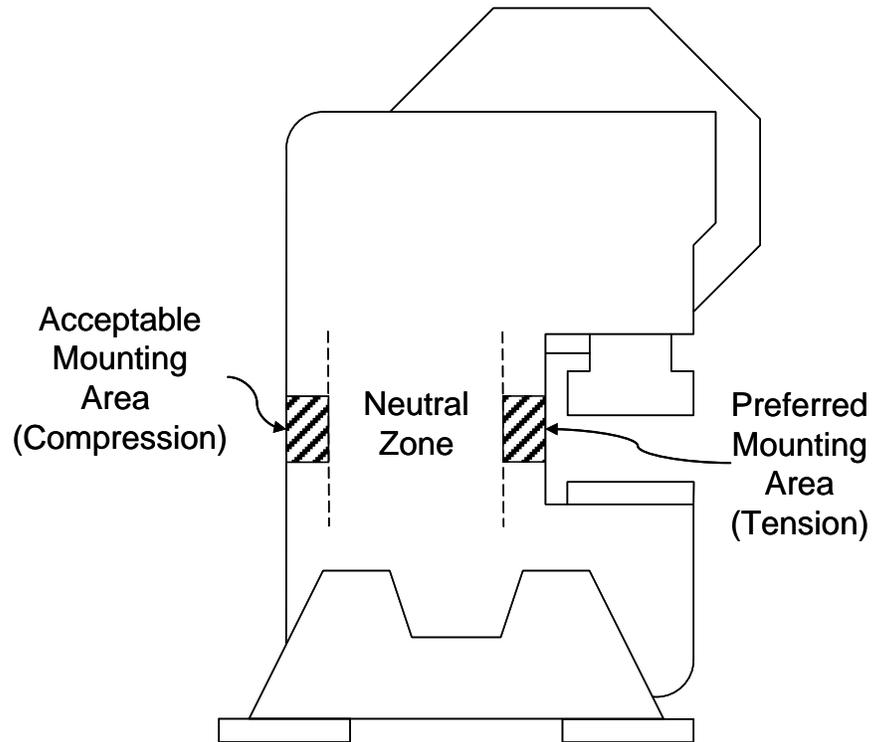
Figure 66: "C" Frame Machine Gage Locations
