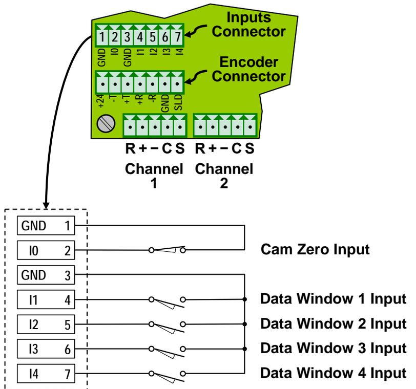
Figure 63: Inputs driven by Cam Zero and Data Windows
