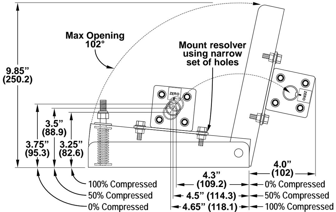
Figure 56: Spring Base with 5100-11 Encoder Dimensions
