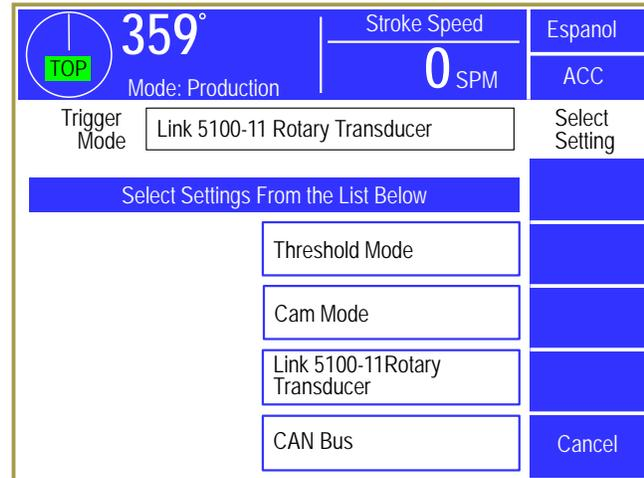
Figure 27: Selecting Trigger Mode
