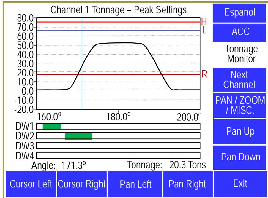
Figure 75: Load Cell Hit with Bad Tie-Rod Tension
