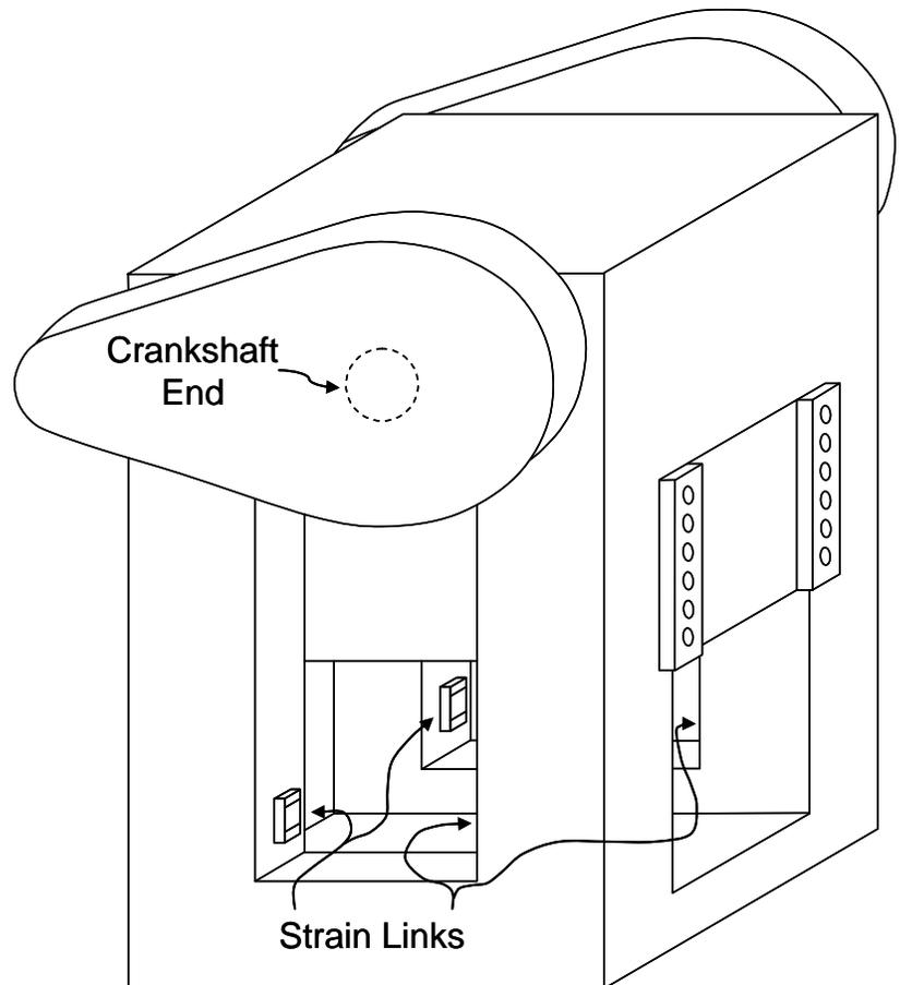
Figure 69: Solid Frame Machine Gage Locations
