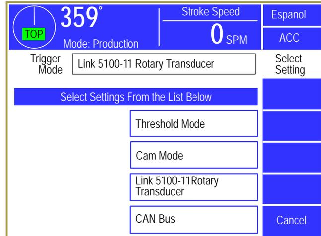
Figure 27: Selecting Trigger Mode
