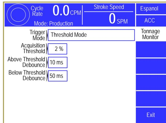
Figure 28: Threshold Trigger Mode Config
