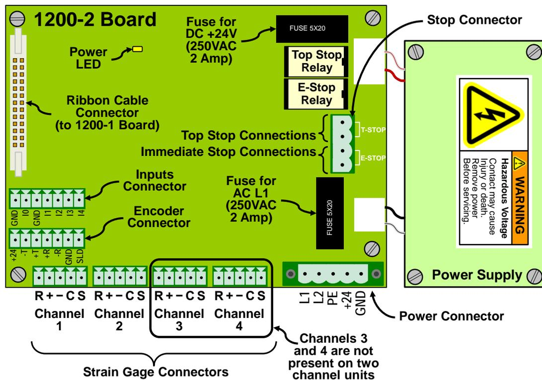
Figure 59: 1200-2 Board Connections
