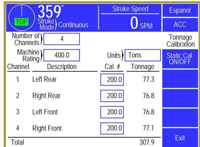
**Figure 36: Tonnage Monitor Tonnage Calibration Screen**
