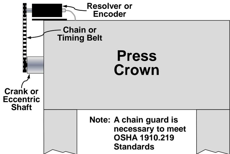
Figure 53: Resolver Mounting to Shaft
