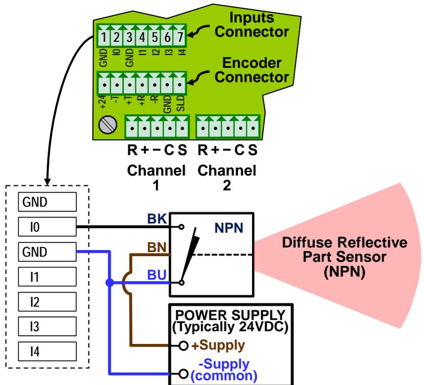
Figure 64: Inputs driven by NPN sensor
