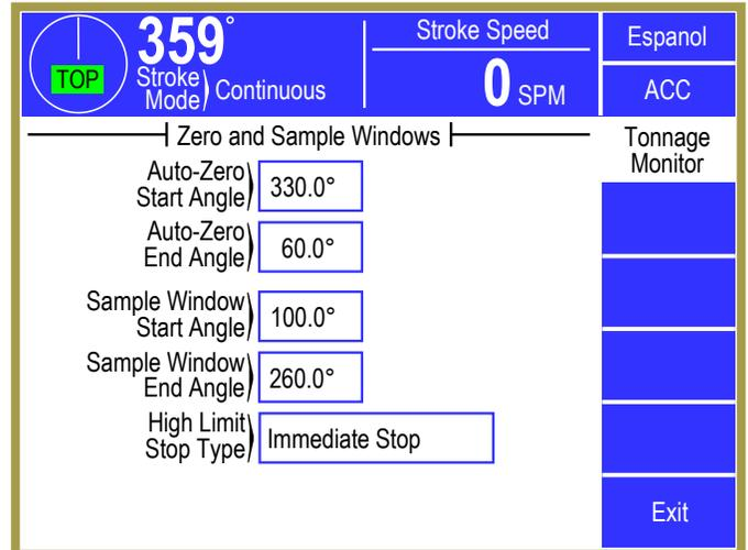
Figure 13: Zero and Sample Windows Configuration Screen
