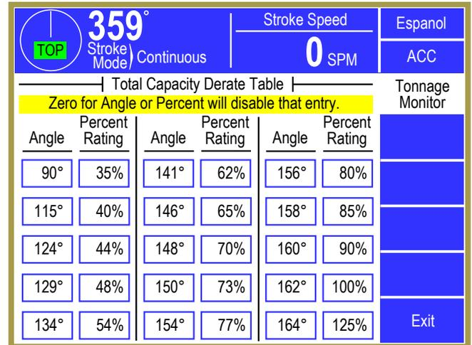
**Figure 15: Tonnage Monitor Total Capacity Derate Screen**
