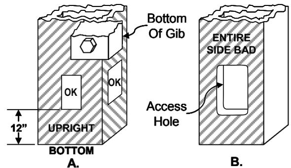
Figure 21 shows areas to avoid on the uprights of straight side machines of tie rod construction. The cross-hatched areas should be avoided.
