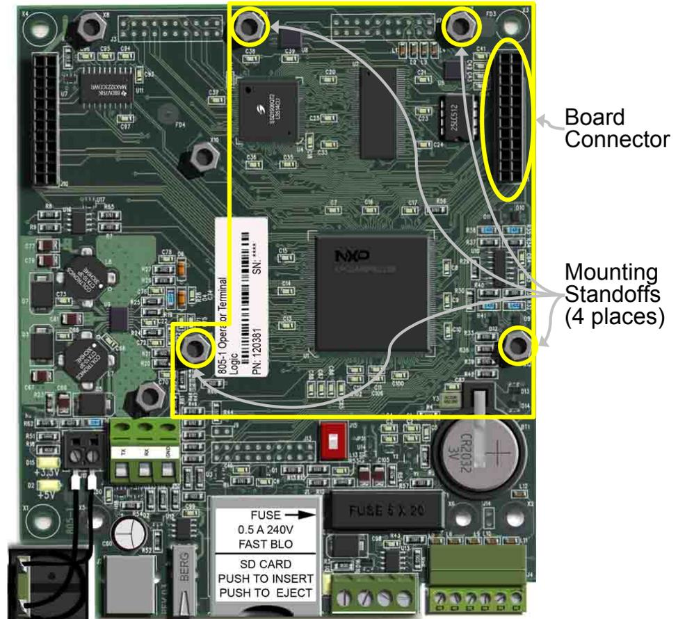
Figure 17: Mounting Location of Board in the OIT
