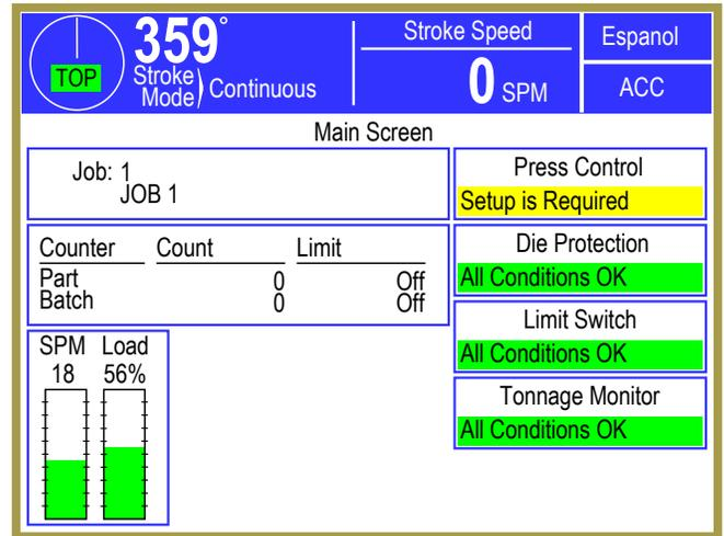
**Figure 3: Operator Terminal Main Screen**
