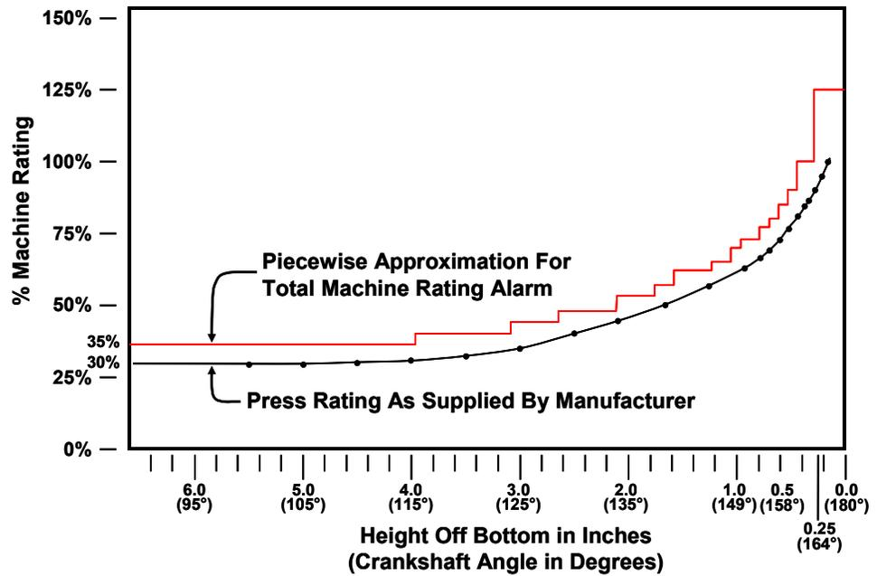
Figure 16: Example Tonnage De-rate Curve
