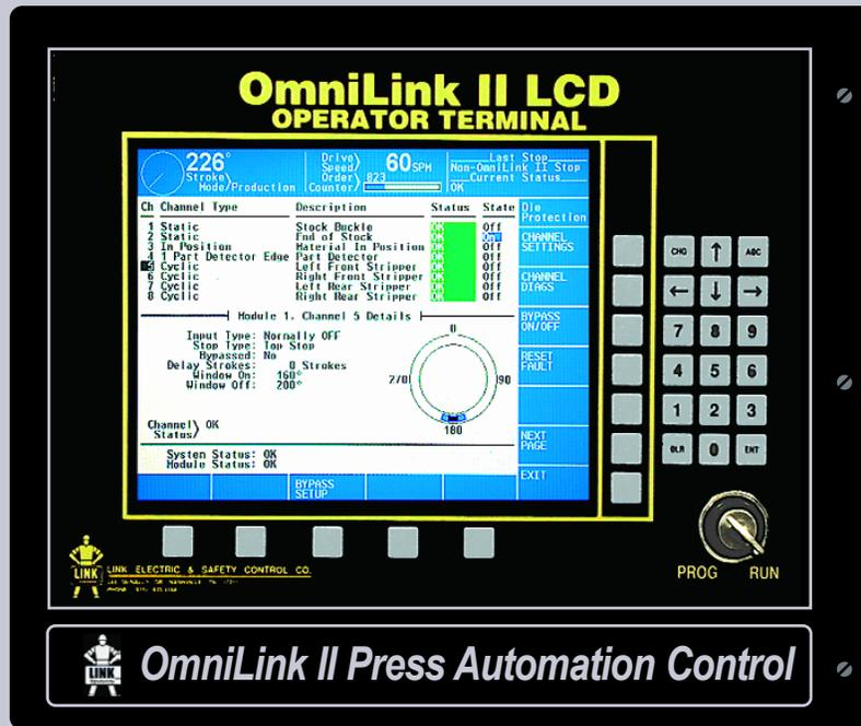
*The most advanced modular press automation system available with control, sequencing, monitoring, job storage, diagnostic and communication functions to increase productivity and quality in press production processes to new levels for global competitiveness.*
