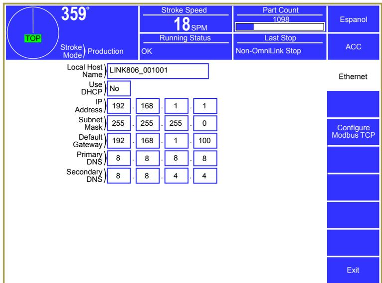
**Figure 52: Ethernet Configuration Screen**
