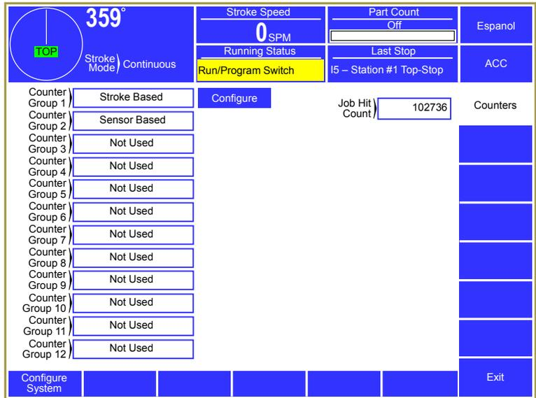
**Figure 16: Counter Configuration Screen**
