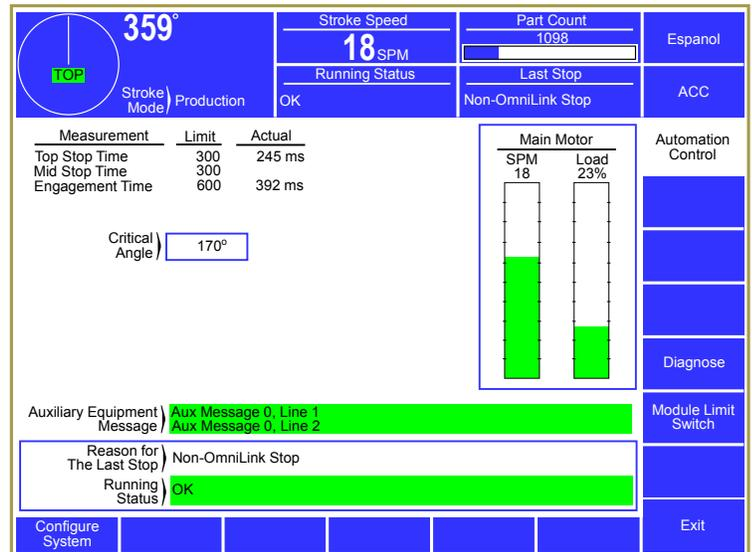
Figure 24: Automation Control Screen (Mechanical Press)
