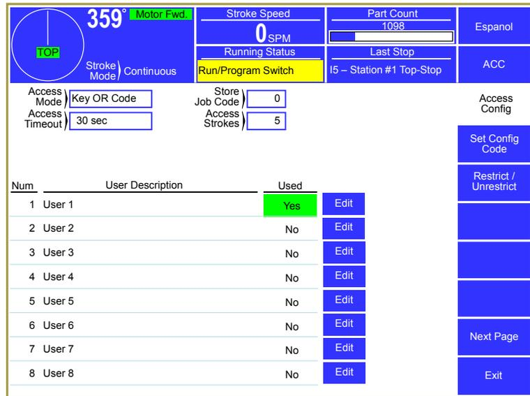
**Figure 47: Access Configuration Screen**
