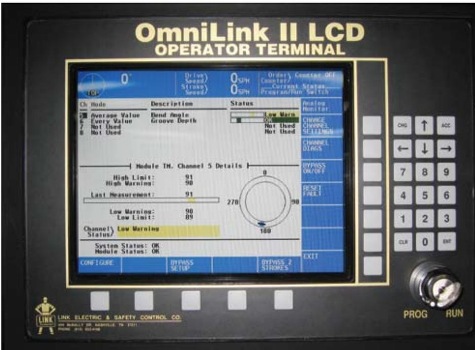
A control from Link Systems integrates in-die-measurement setup and programming. (Courtesy of Link Systems)
