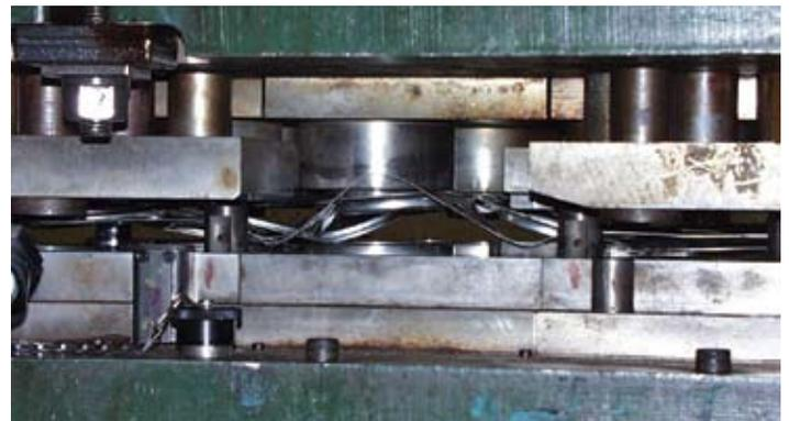
A press-save at Bachman Machine showing a short-feed condition. The die-protection control on the press stopped motion before a die crash occurred. (Courtesy of Bachman Machine)
