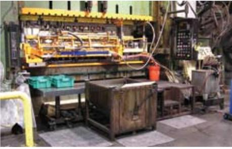
Bachman Machine uses sensors on all critical press operations, including the progressive-transfer operation above. (Courtesy of Bachman Machine)
