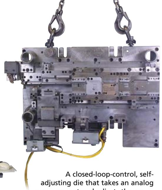
A closed-loop-control, self-adjusting die that takes an analog measurement and adjusts the servomotor automatically, if necessary, while the die is running. (Courtesy of Bachman Machine)
