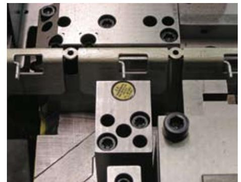
An analog sensor in a self-adjusting die. (Courtesy of Bachman Machine)
