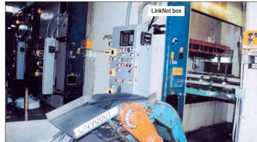
Upgrading presses at Electrolux included installing new controls such as the OmniLink shown here on one of the Komatsu presses on the chassis line. Note the LinkNet connection box wired to the control—every press in the pressroom carries one of these boxes, daisy-chained through the plant to deliver production data to an office computer.
