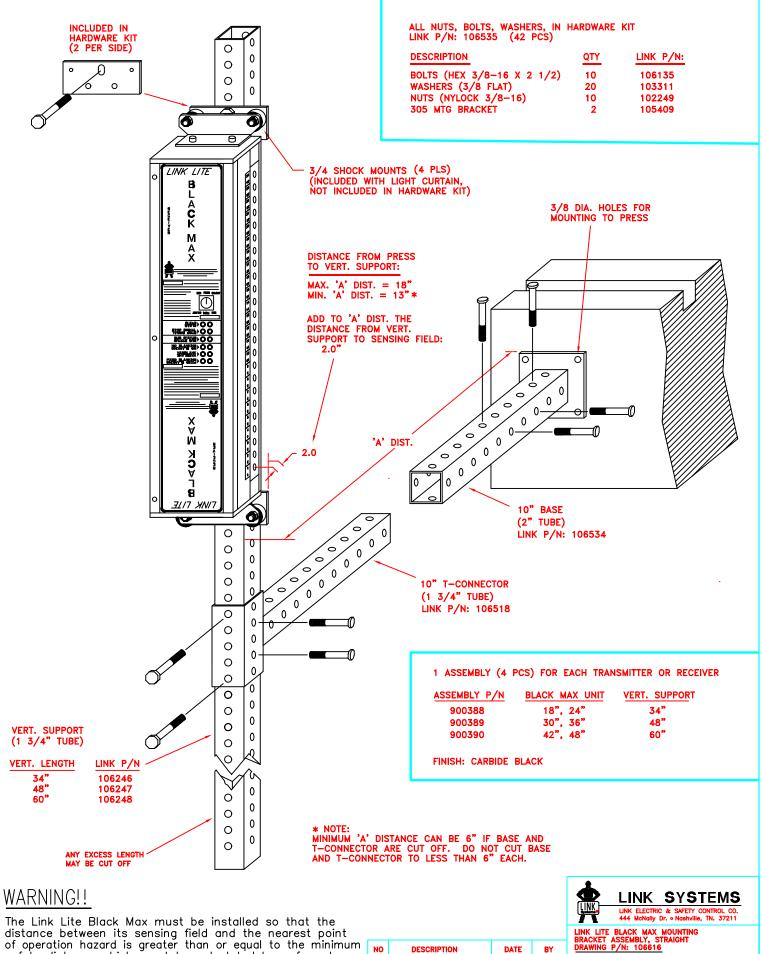
distance between its sensing field and the nearest point of operation hazard is greater than or equal to the minimum safety distance which must be calculated by a formula specified by OSHA and ANSI. See latest editions OSHA 1910.217, ANSI B11.1 and B11.9.
