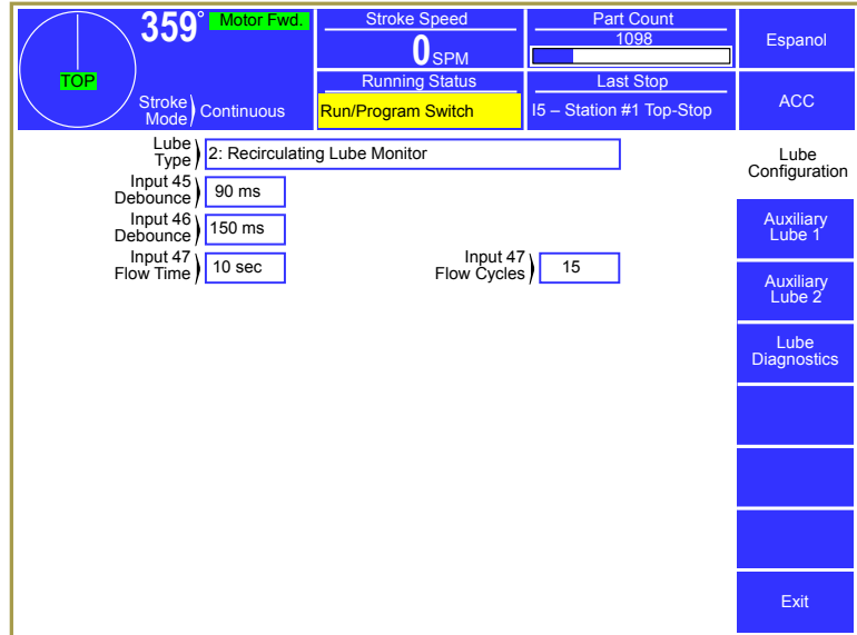
Figure 69: Lube System Configuration Screen (Type 2)
