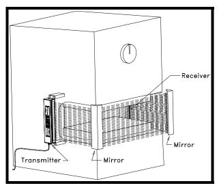
**Figure 3.11:** Example of three sided point of operation guarding on C frame press.
