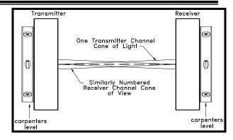
**Figure 3.20b:** Black Max transmitter and receiver in alignment from front view.
