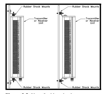
**Figure 3.5:** Use of rubber shock mounts.
