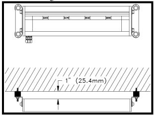
**Figure 3.9a:** Example of remote segment Black Max unit mounting.
