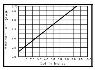
**Figure 3.2:** Graphical Representation of penetration depth factor,  $D_{pf}$ , vs. minimum object sensitivity.
