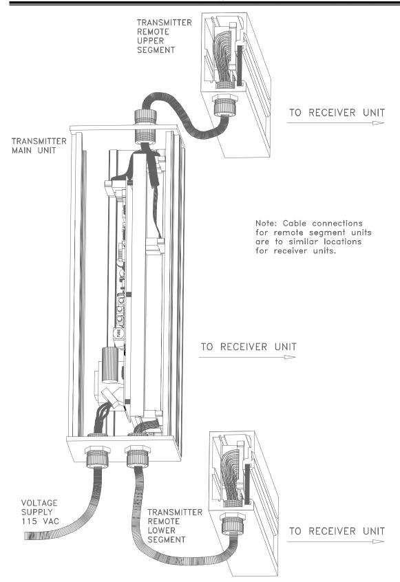
Figure 3.18: Use of two remote segment units with main transmitter.
