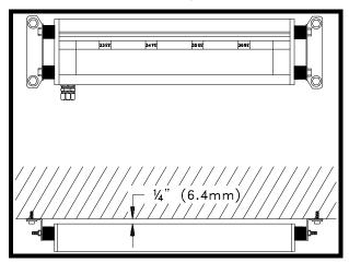
**Figure 3.9b:** Alternate remote segment Black Max unit mounting.
