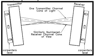
**Figure 3.20a:** Black Max transmitter and receiver out of alignment from front view.
