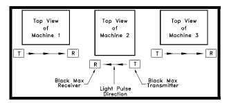
**Figure 3.4:** Mounting scheme to minimize crosstalk.
