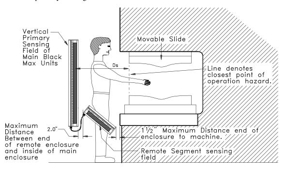
**Figure 3.8:** Remote segment Black Max units oriented at an angle to sense a person between the primary sensing field and the hazard.
