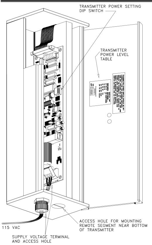
Figure 3.19: Location of the transmitter power level switch and power level table.
