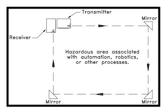
**Figure 3.12:** Top view of four sided perimeter guarding application.
