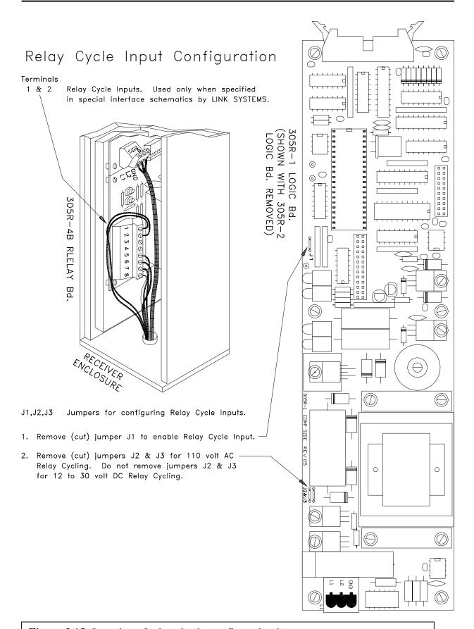
**Figure 3.15:** Location of relay check con-figuration jumpers.
