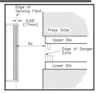
**Figure 4.2:** Illustration of Minimum Safety Distance Measurement
