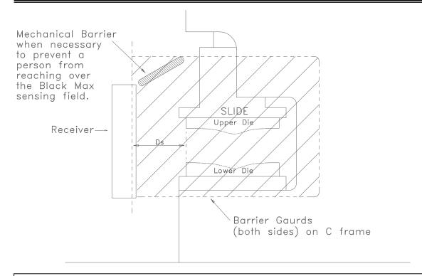
**Figure 3.23:** Illustration of barriers installed to prevent someone from reaching over the top of a Black Max sensing field or through the openings of a C frame machine.
