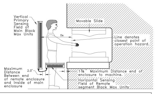
**Figure 3.6:** Horizontally mounted remote segment Black Max units to detect a person inside the main sensing field.
