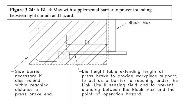
Figure 3.25: Example of a Black Max on a press brake with supplemental barriers.
