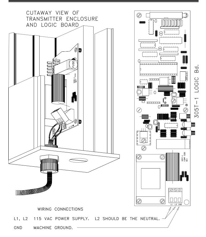
**Figure 3.13:** Location of transmitter power connector.
