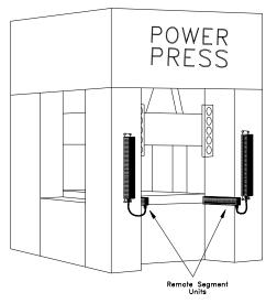
**Figure 3.7:** Remote segment Black Max units mounted between columns of straight side power press to detect a person standing inside the primary sensing field.
