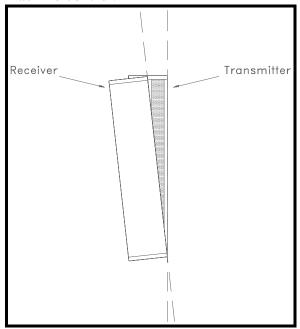
**Figure 3.22a:** Transmitter and receiver out of alignment from side view.
