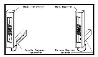
**Figure 3.10:** Mount main and remote transmitter and receiver units on the same respective sides.
