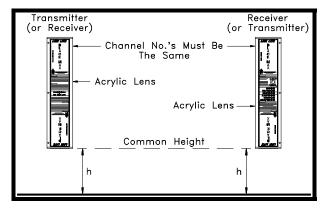
**Figure 3.3a:** Front view of transmitter and receiver units mounted at a common height.
