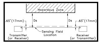
**Figure 3.3b:** Top view of transmitter and receiver units.
