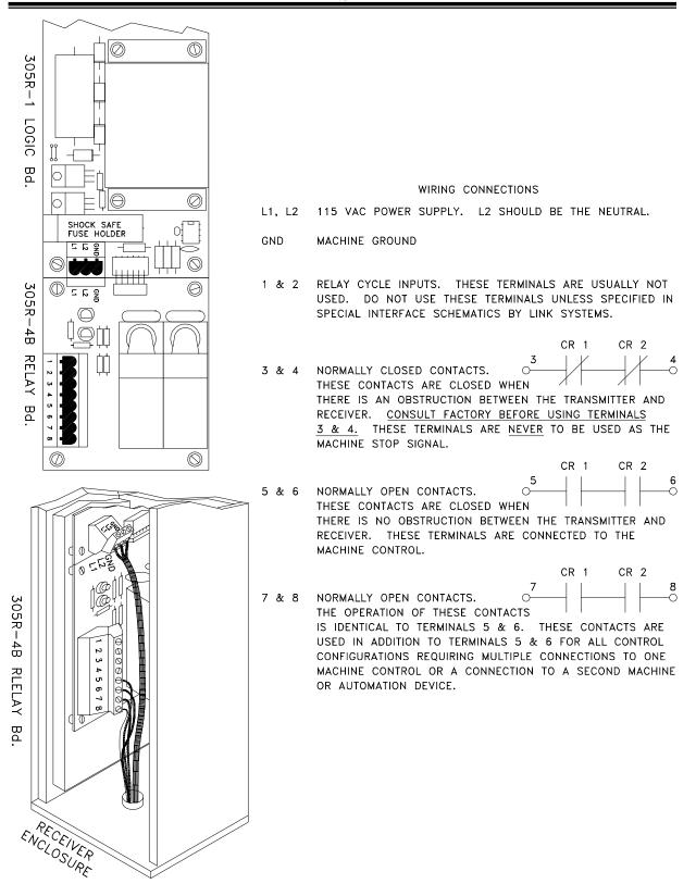
**Figure 3.14:** Power and relay connections for Black Max receiver.
