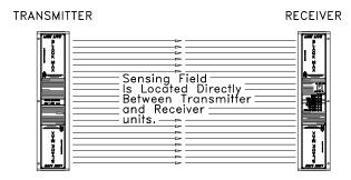
**Figure 4.1:** Illustration of sensing field location between main Black Max transmitter and receiver units when no blanking is used.
