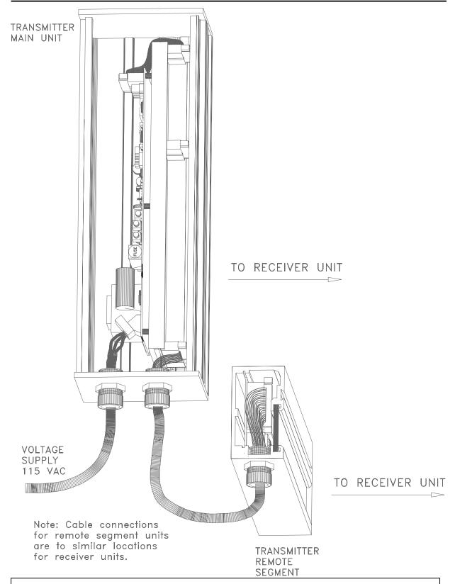
Figure 3.16: Use of remote segment at bottom of main transmitter.
