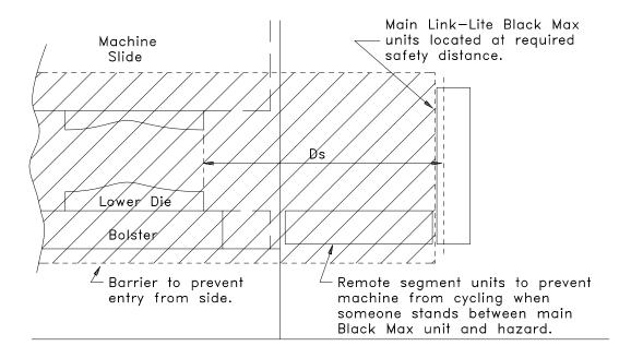
**Figure 3.26:** Use of Black Max remote segment units in the horizontal position to protect inside primary sensing field, and barriers to prevent entry from the side.
