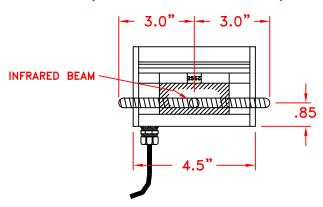
TRANSMITTER or RECEIVER side view
