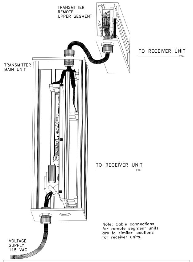
Figure 3.17: Remote segment unit used at top of main transmitter.
